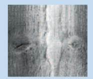
The intensity image of a board to the left and the scatter image (Tracheid) to the right. Note how the knots in the scatter image appear much darker than in the intensity image, thus making the knot identification much easier and more robust.
